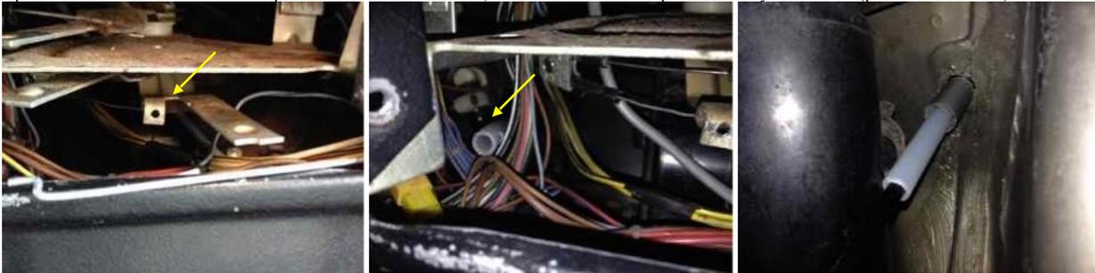
Behind the front grille to the left of the radiator is a 1/2" blind rubber grommet blocking a hole in the van firewall. Remove this grommet to expose the hole in the bodywork there that the control cable will go thru (shown above right with poly tube and cable).
