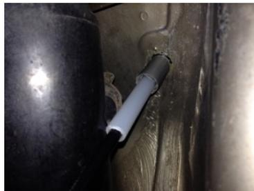
Behind the front grille to the left of the radiator is a 1/2" blind rubber grommet blocking a hole in the van firewall. Remove this grommet to expose the hole in the bodywork there that the control cable will go thru (shown above right with poly tube and cable). Insert the poly tube into the hole you removed the blind grommet from. You need to maneuver the tube thru the space under the dash until the tube is aligned with the 3/8" hole you drilled.
