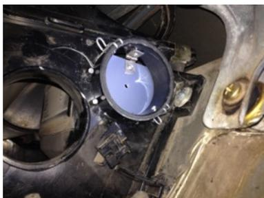
If the hole is too large and the valve is too loose a fit to stay in place on its own, use two of the #6 x 1/2" hex-head sheet metal screws thru the wire ears to secure it. These might not be needed at all if the fit is tight enough, use your own judgment. The screws will self-drill if you use a power screwdriver, otherwise you can pilot drill with the 1/8" bit thru the wire ears. Tighten the screws very gently as the plastic will easily strip out.
