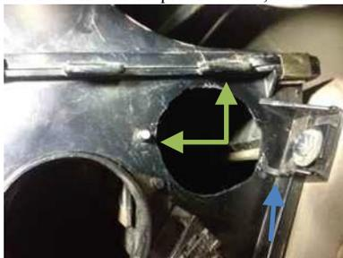
Positioned so, make a center punch mark at the bottom forward (lower-right as you are looking at it) corner of the square, then remove the square. Drill a 1/8" pilot hole at the punch mark, then cut out a circle with the 2 1/8" holesaw (your hole will probably look much better than the one in the picture, that hole was enlarged by hand after I cut it too small the first time!).
