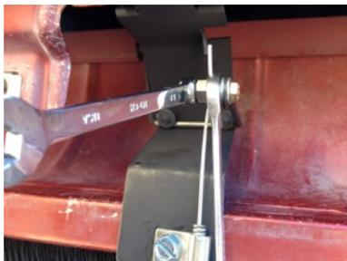
Push upward against the bellcrank to hold the door tightly closed, and using an 8mm open end wrench to hold the swivel barrel, use a 7mm wrench to tighten the M4 setbolt until it just begins to grip the cable wire. Pull the cable wire upward to be sure the knob inside is all the way in, and holding that wire position make sure the bellcrank lever is pushed as far upward as it can go and the inlet door is pressed closed. Tighten the M4 setbolt to hold the cable wire firmly, as shown at left.
