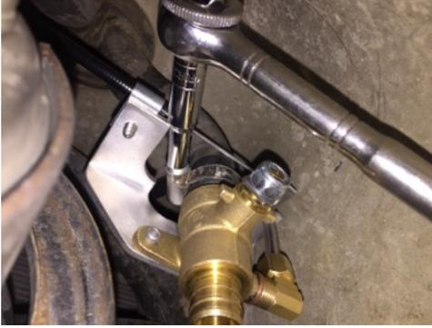
fitting. If the tube becomes sticky to the touch, it's too hot and will be too soft to insert the barb, so let it cool and try again. After the tube is slid all the way onto the barb, let it cool, then move the crimp clamp over the barb and compress it gently with pliers or end nippers.
