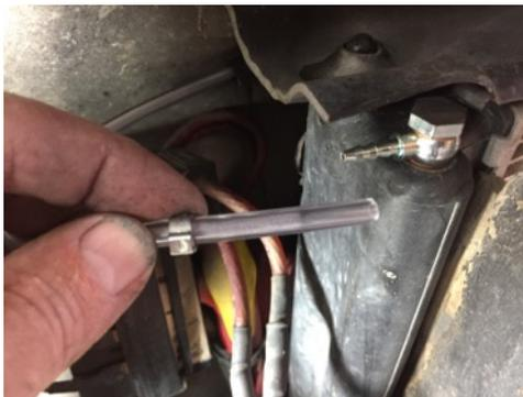
Remove the old radiator bleeder bolt. Install the check valve bolt, banjo end fitting and copper washers as shown at left. Tighten moderately, it doesn't take much torque to seal this type of fitting, and there is a danger of stripping the threaded insert in the radiator by overtightening. Also, the copper washers will seal again and again, there is rarely any need to replace them unless the fitting has been overtightened.
