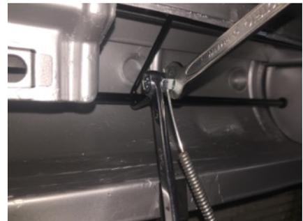
Gently push the bellcrank's cable attachment arm up and down to open and close the door, everything must move freely. Do not bend the bellcrank to force the door closed, instead find out where the drag is and make adjustments as necessary.
