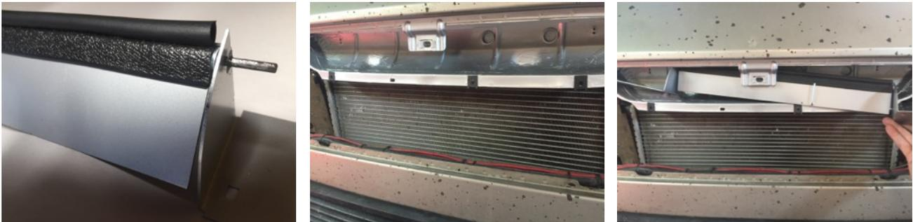
Install three of the (4) clip-nuts over the furthest left, second from left, and furthest right holes in the bottom edge of the cabin air scoop, as shown above center.
