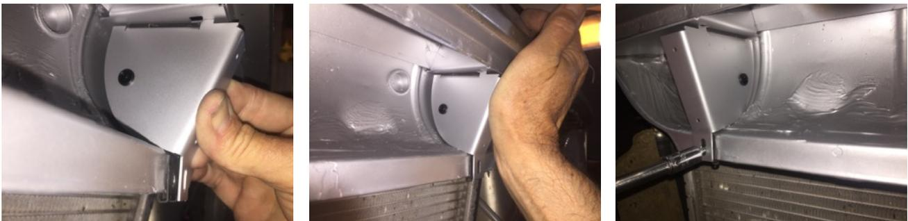
The jamb piece should be held in position where its forward long edge pushes up against and runs along the upper rim of the grille opening, just covering it from below.
