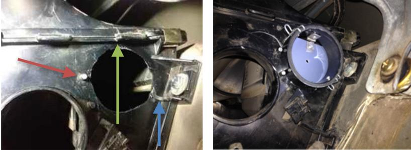
Cut a piece of thin cardboard exactly 1 3/16" square as a pilot hole marking guide. Place the paper square flat onto the end face of the air distribution box, top edge butted up against the rim of the air box cover seam (green arrow far left picture), and left side of the rectangle butted against the embossed pin which is colored white (red arrow).
