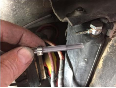
Remove the old radiator bleeder bolt. Install the hollow banjo bolt, banjo end fitting and copper washers as shown at left. It takes only light torque to seal this type of fitting, and the copper washers will seal again and again if tightened moderately, so it's OK to loosen the banjo bolt repeatedly to aid coolant filling as you normally would.
