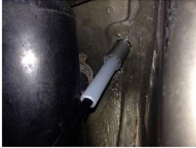
Behind the front grille to the left of the radiator is a 1/2" blind rubber grommet blocking an existing hole in the van firewall. Remove this grommet to expose the hole in the bodywork there that the control cable will go thru (shown at left with poly tube and cable). Insert the poly tube into the hole. You need to maneuver the tube thru the space under the dash until the tube is roughly aligned with the 3/8" hole you drilled.
